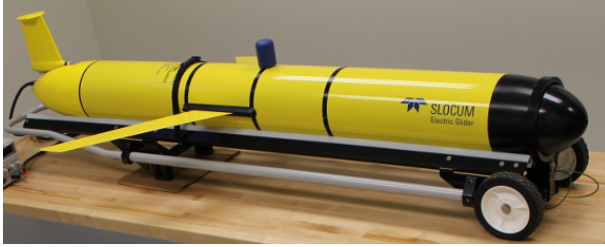
Figure 1. One of our Slocum Gliders equipped with a double payload bay. The glider is 180 cm long and weighs around 70 kg.
